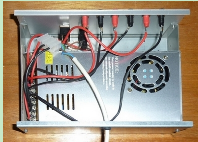
Crimp soldered and heat shrunk on mains neutral
