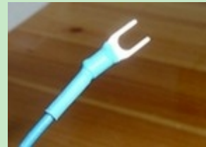
Crimp soldered and heat shrunk on mains neutral
