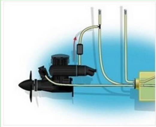
Figure 2: This is the Uniflow 3-line pressurized system. Note the check valve above the muffler. It permits pressurized gas to flow in only one direction into the fuel tank. Note that the pressure line carrying exhaust has a clunk that is next to the feed line clunk. Both clunks are in the same relative position with respect to the mass of fuel. This takes the pressure differential noted in the first illustration out of the equation.
