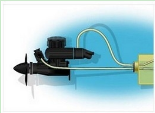
Figure 1: This conventional 2-line pressurized system is used on most models. Note that a pressure line carries exhaust pressure from the muffler to the air pocket in the top of the tank. A pressure differential between that applied to the pressure line versus the feed line leading to the carburettor varies as the amount of fuel decreases and as the aircraft changes attitudes or goes inverted. The Uniflow system eliminates this variance.
